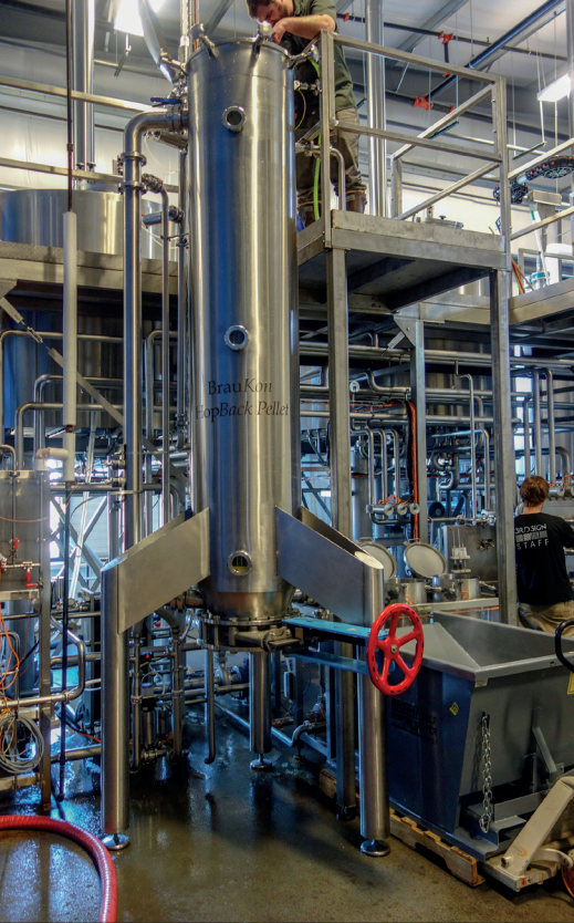
HopBack Pellet retrofit installation for 60 kg (USA)
