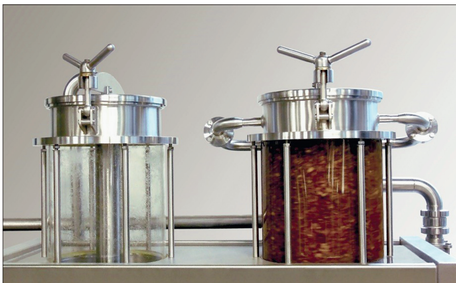
Hop dispenser including spice extraction integrated into the whirlpool (USA)
