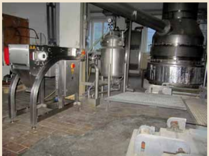
Fig. 3 The compressed hop separation machine (left) with a rectification wort boiling system (right) at Alpertsbacher Klosterbräu
