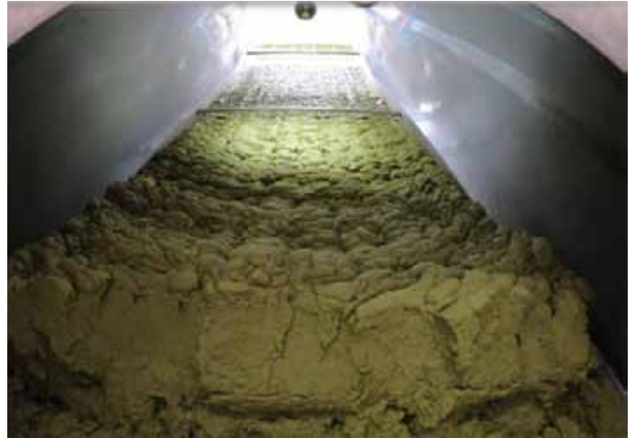
Fig. 4 Bottom discharge of hop trub
