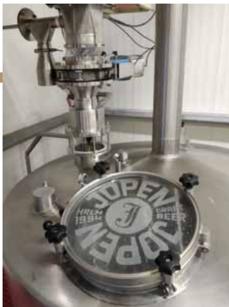
Fig. 5 The recently installed AlloySius grist hydrator and GentleMix agitator help achieve a thoroughly mixed mash, free of clumps
