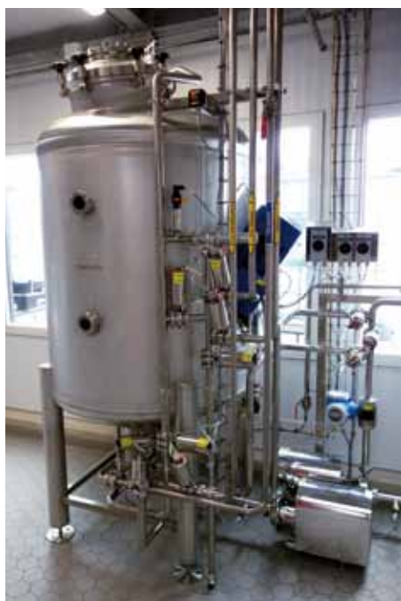
Fig. 2 The HopGun Pro, integrated in a dry hopping loop, allows for automation of the dry hopping process
