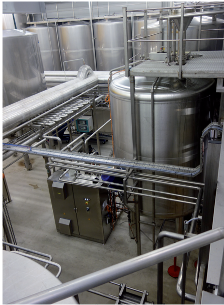
Fig. 4 Dispersion and dosage system unit for batch sizes of up to 1000 kg
