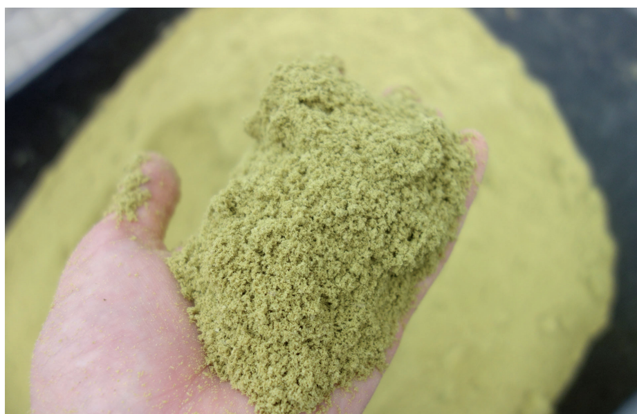
Fig. 3 Hop solids separated after extraction (35 % dry substance)
